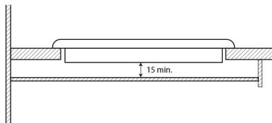
Gently insert hob into cut out, allowing clips to hold the hob in place.
