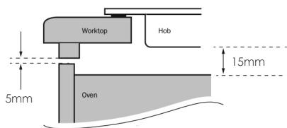
If the installation is not above an oven and the underside of the hob is accessible, a wooden shield is required to be installed at least 15mm below the underside of the hob unit.
