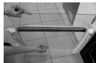
**Remove the centre glass taking care to support the weight of the glass when removing and fitting**
