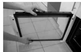
**Open the lower door and lift out the inner door glass**
